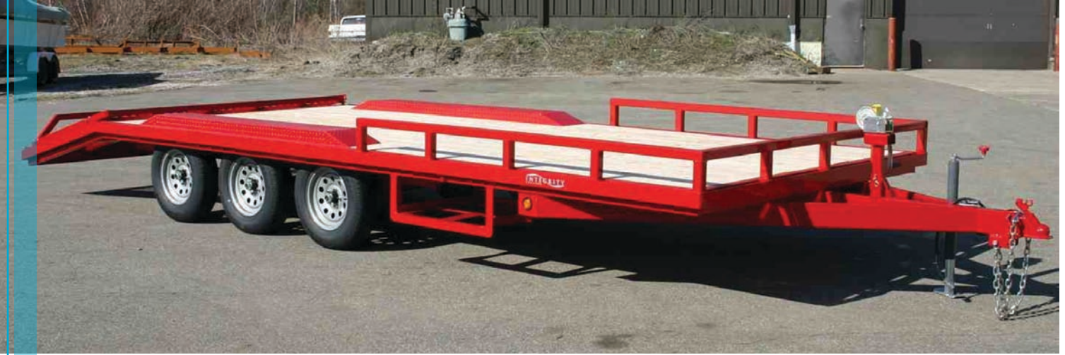
97.5" x 24' Deckover Utility Trailer, 9,900 GVW (Optional Equipment Shown)
